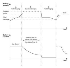
Figure 1-4 Battery changing stage
