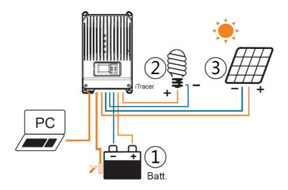
Figure 2-2 Connection Diagram
