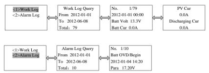
Work Log and Alarm Log could be browsed in this interface, the operation is as follows:
