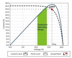
Figure 1-2 Maximum Power Point Curve
