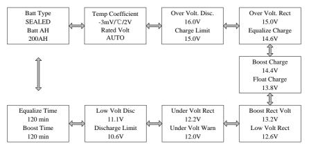
You should input the user password (see above) before setting the parameters. In setting mode, all the parameters can be modified. And will immediately effect when saved. The detail and value range of control parameter are shown in the tables below:
