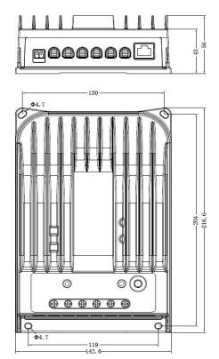
Tracer2215BN Dimensions in Millimeters
