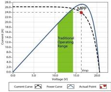
Figure 1-2 Maximum Power Point Curve
