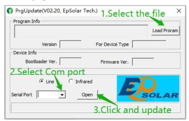
**Step5:** Click the "Load Program" button to select the upgrade file according to the specified controller, such as ST\_TcerAN\_V200.prg.
